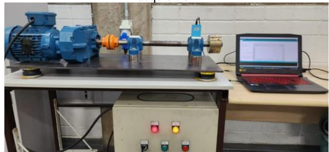
Figure 3 – Sensor connected to the bearing during an acquisition
